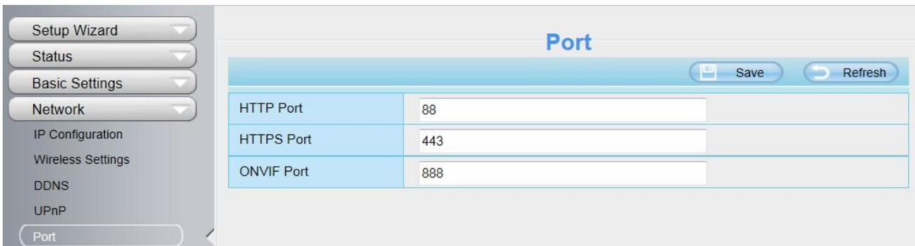
4. If the UPnP of the router has been enable, you do not need to perform following steps. Otherwise, you need to select one of the following methods to configure port forwarding on your router. For these steps, we will be using the TP-LINK brand wireless router as an example.
