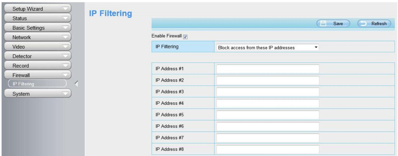
Enable firewall, If you select Only allow access from these IP addresses and fill in 8 IP addresses at most, only those clients whose IP addresses listed in the Only allow access from these IP addresses can access the Network Camera. If you select Block access from these IP addresses, only those clients whose IP addresses are in the IP list cannot access the Network Camera.
