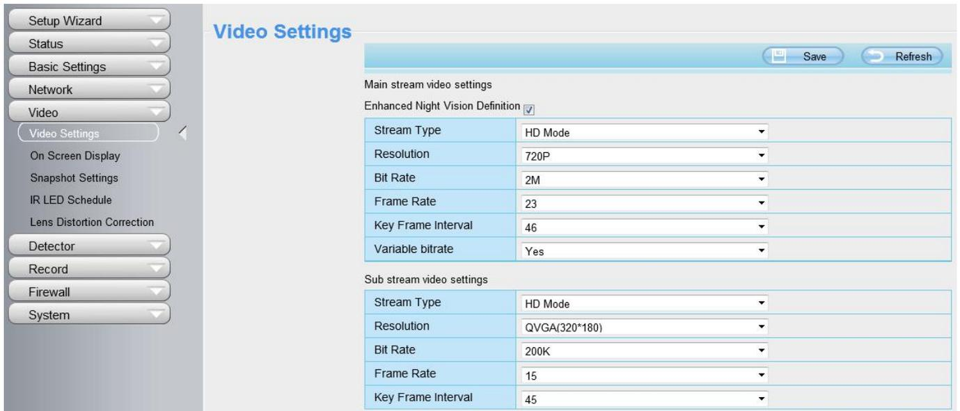
**Enhanced Night video Definition:** The camera will automatically drop the frame to extend the recording time in the night.
