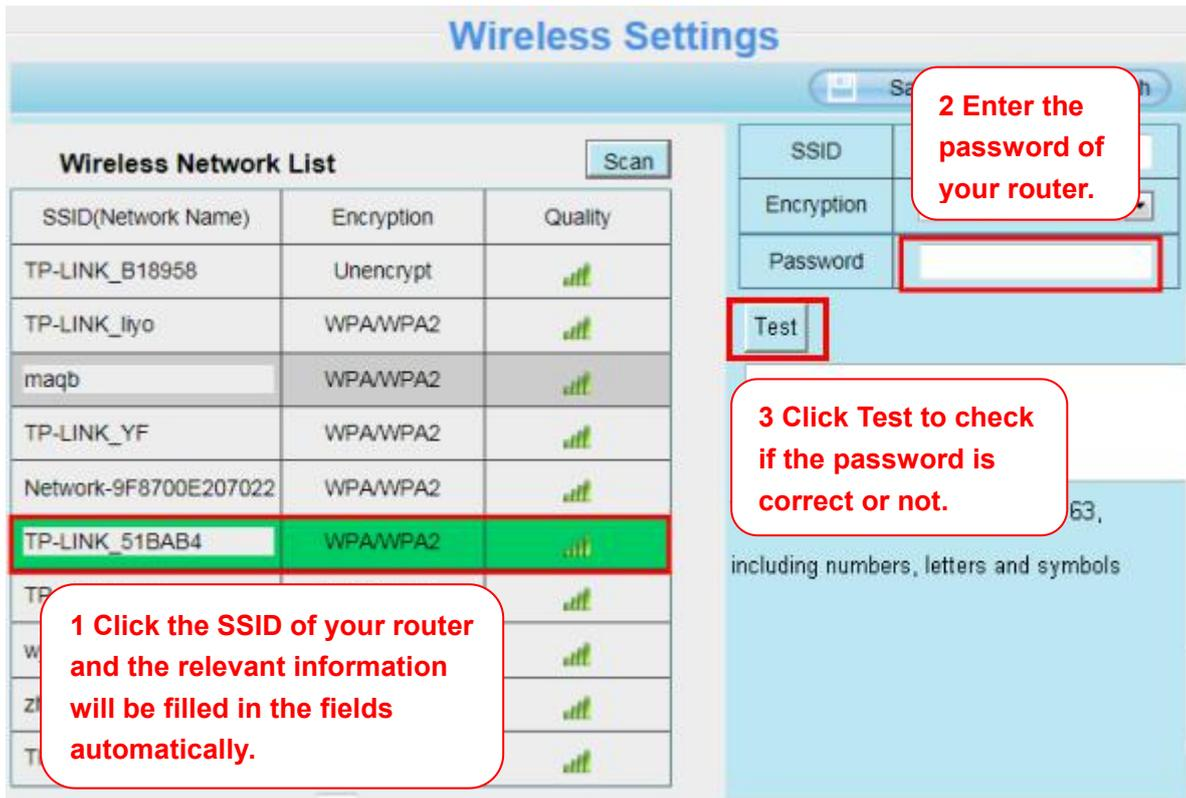
**Step 3:** Please click on the **Save** button after all settings have been entered and disconnect the network cable. Never shut down the power of the camera until the IP camera is able to connect to the wireless network.
