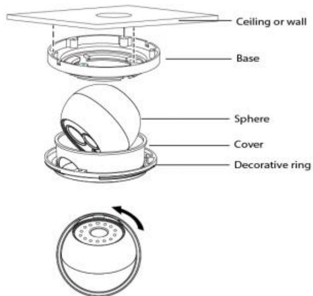
3. Assemble the sphere, cover, and decorative in order, set the angle of the camera viewing area.
