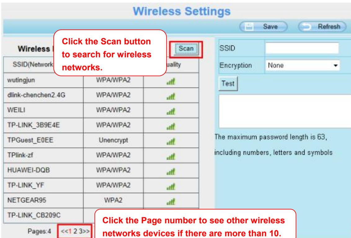
**Step 2:** Click the SSID (name of your router) in the list, the corresponding information related to your network, such as the name and the encryption, will be filled into the relevant fields automatically.
