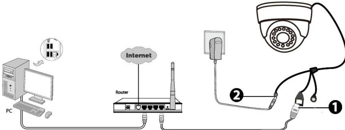
1. Connect the camera to the LAN network (Router or Switch) via ethernet cable.
