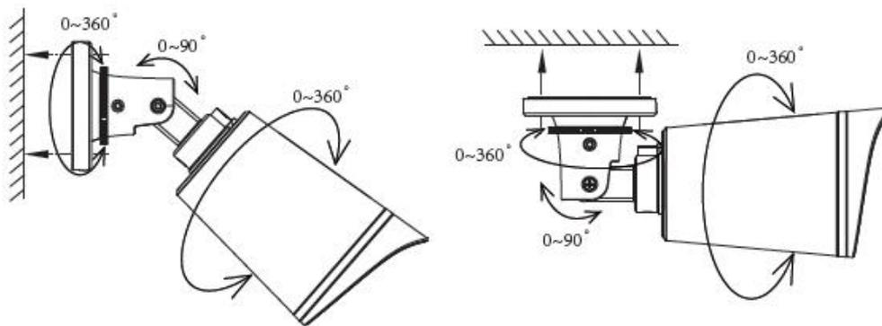
Fixate the camera on your preferred location and use screws to mount it. We have provided screws in the Packaging.
