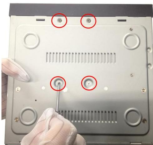
4. Re-install the cover of the NVR and fasten screws.
