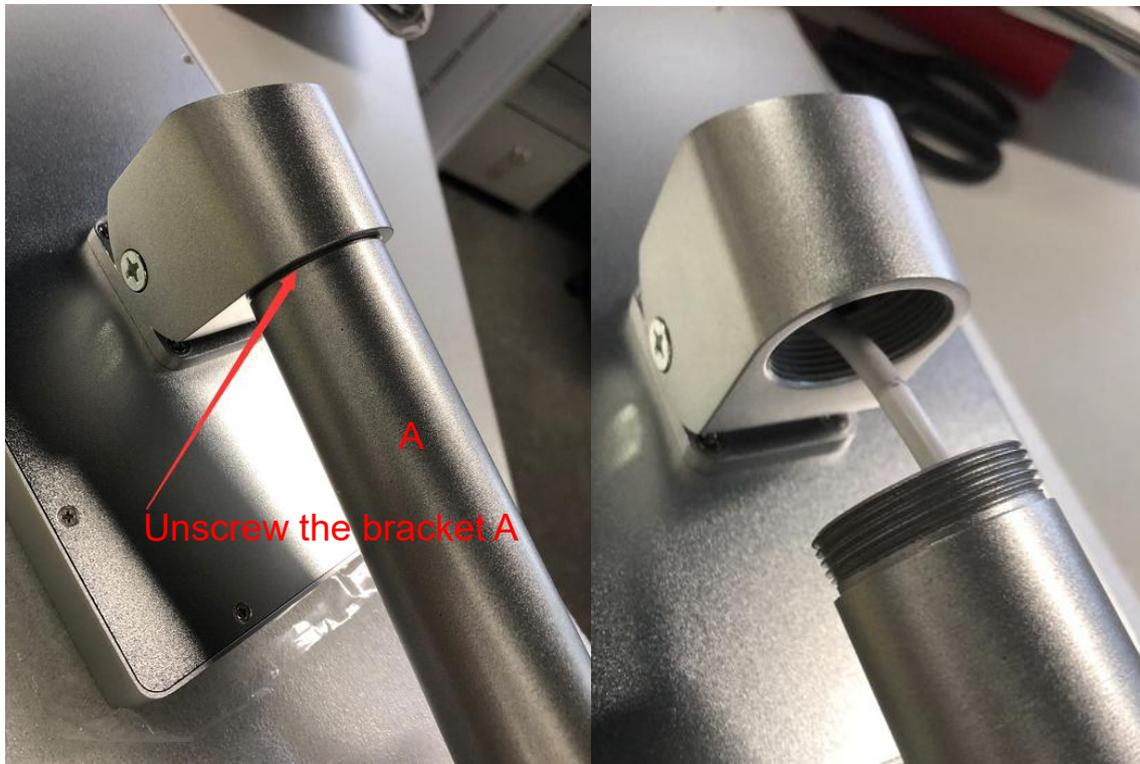
2. Take the tail wire out of the bracket, as shown in the figure below.
