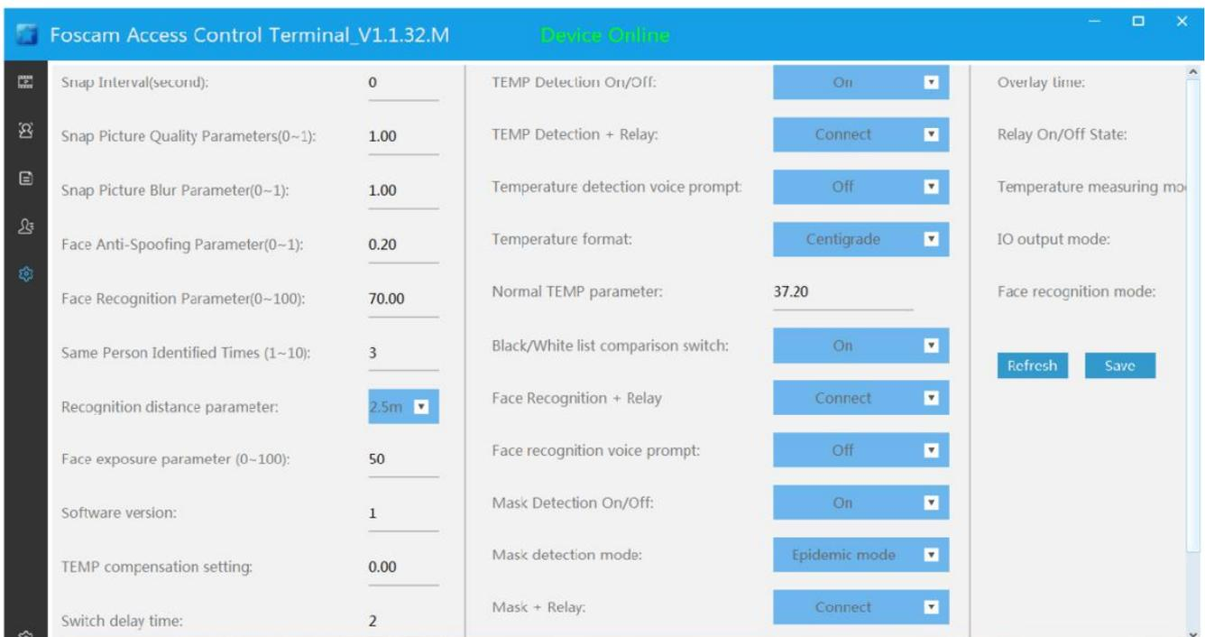
**Snap Interval:** set the face capture time interval to avoid repeated capture of pictures in a short time.
