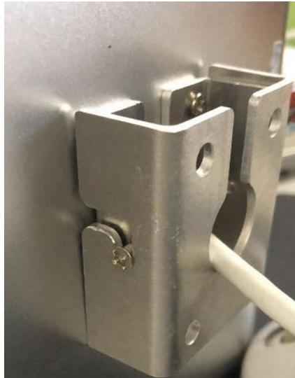
10. Finally, use a screwdriver to tighten the side screws to prevent falling.
