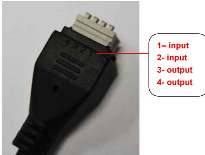
This camera supports I/O alarm, you can go to **Settings-Alarm - I/O** page to configure it.
