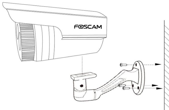
Step 1: Screw the mount on the wall with the 3 screws provided.
