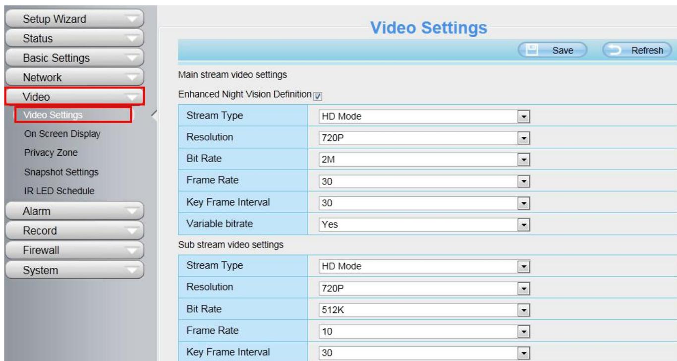
**Enhanced Night video Definition:** The camera will automatically drop the frame to extend the recording time in the night.
